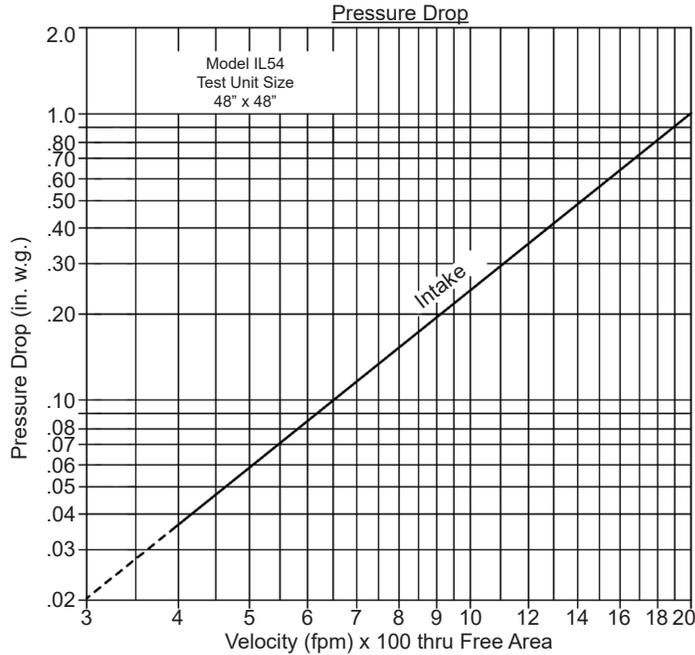
Intake air converted to standard air density.
